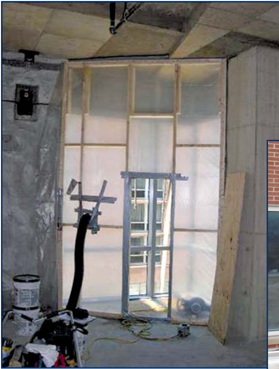
Photo 10 – Interior isolation chamber and test apparatus for a pressurized E 1105 test.
