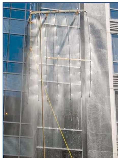
Photo 9 – ASTM E 1105 spray rack in use on the exterior of an aluminum and glass curtain wall.
