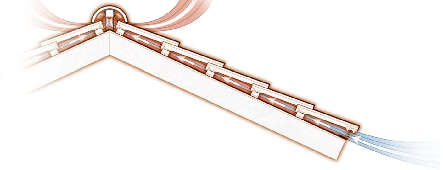
Figure 2 – Above-sheathing ventilation (ASV).
