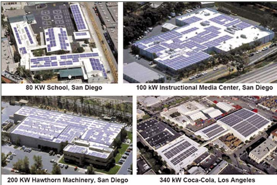
Figure 4 – Solar Integrated Technologies' thin-film laminated roofs.
