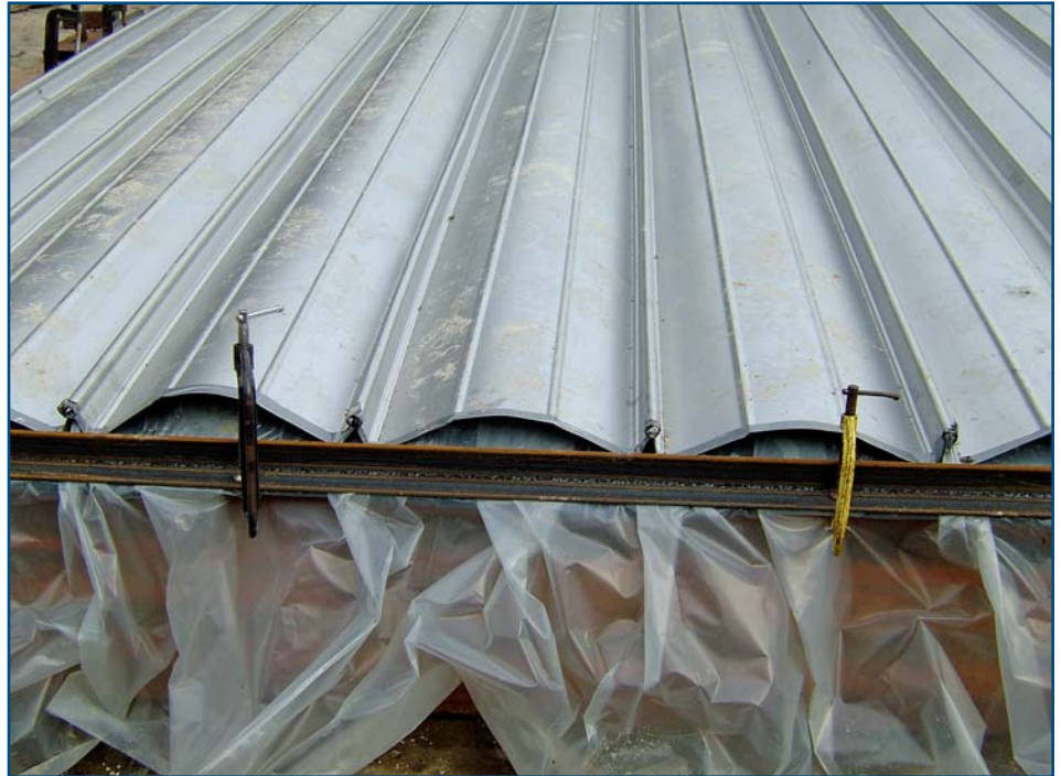
Photo 2 – ASTM E-1592 “airbag test” showing how a metal roof panel deflects while resisting a wind load.
