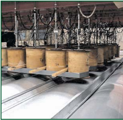
Figure 2 – Research funded by the Metal Building Manufacturers Association (MBA) and the American Iron and Steel Institute (AISI) is ongoing at Mississippi State University. It utilizes electromagnetic fields to more accurately replicate the effects of wind on a roof surface.
