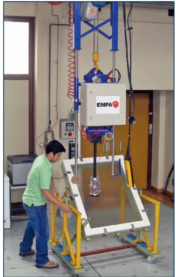
Figure 4 – Test apparatus and tilted steel frame with mounting for a wood-framed window glass.
