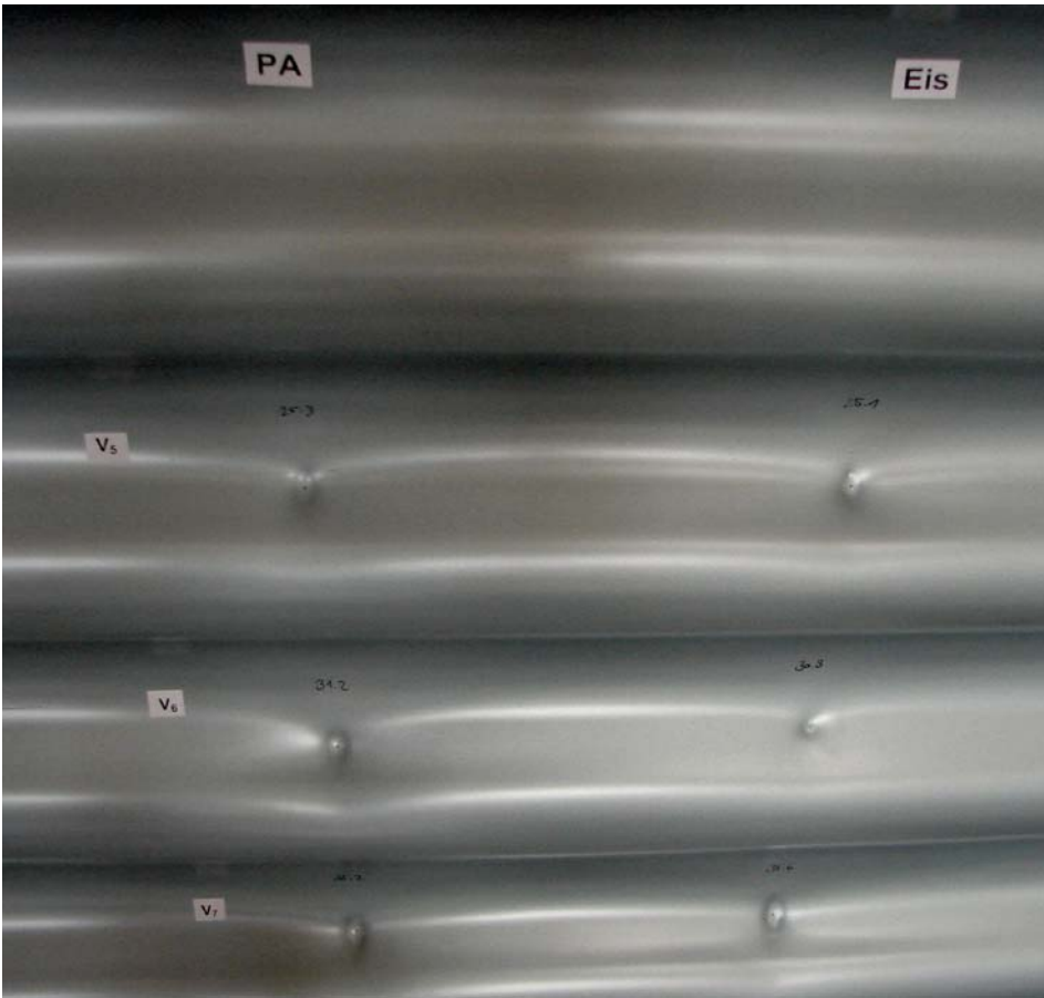
Figure 8 – Indentations caused by 40-mm projectiles. Impact using PA balls (left) and ice spheres (right) at velocities of 26, 30, and 36 m/s.
