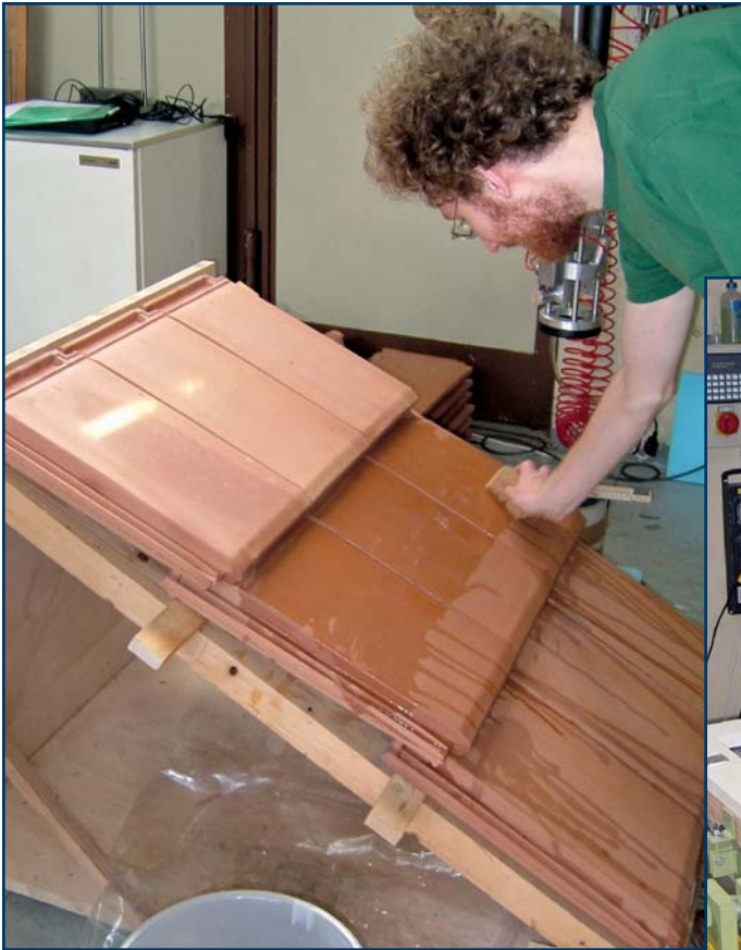
Figure 5 – To condition the clay tile probe before testing, it is moistened three times with a wet sponge.
