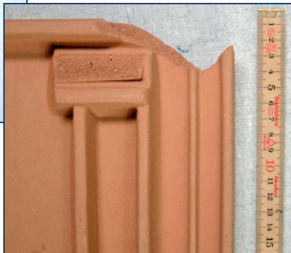
Figure 9 – Fractured clay tiles caused by 40-mm ice spheres: beaver’s tile with center shot at 24.4 J (above); plane tile with corner shot at a kinetic energy of 25.8 J (right).
