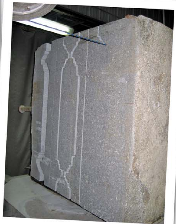
Figure 20 – New granite was custom cut in Canada by computer-guided saws.
