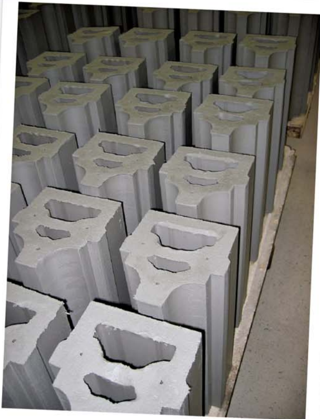
Figures 9A and 9B – New terra cotta was manufactured by extrusion and hand pressing.
