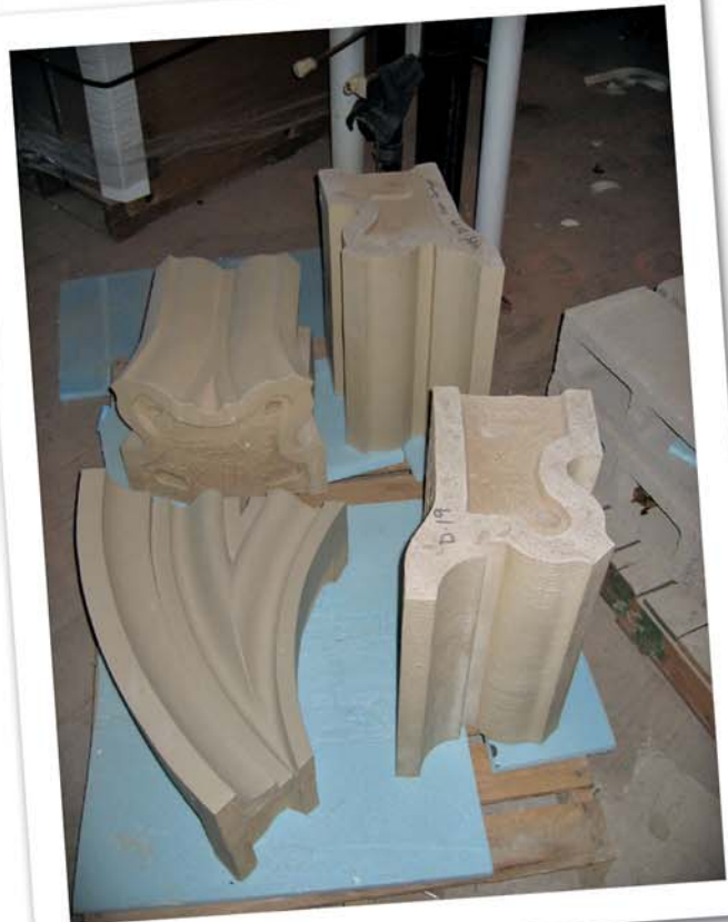
Figures 9A and 9B – New terra cotta was manufactured by extrusion and hand pressing.
