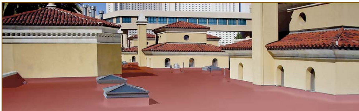
Photo 5 – The cool-colored roof coating on these hotel villas in Las Vegas is decorative and color-stable. The terra cotta cool color was created with infrared reflective (IRR) pigments in a fluoropolymer coating. (Photograph courtesy of Quest Construction Products: United Coatings, Spokane, WA.)
