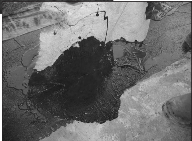
Photo 10 – Fabric embedded in membrane for adhesion test. After the membrane cured, workers pulled the fabric to observe the failure mechanism. The membrane failure occurred within the layers of the membrane.
