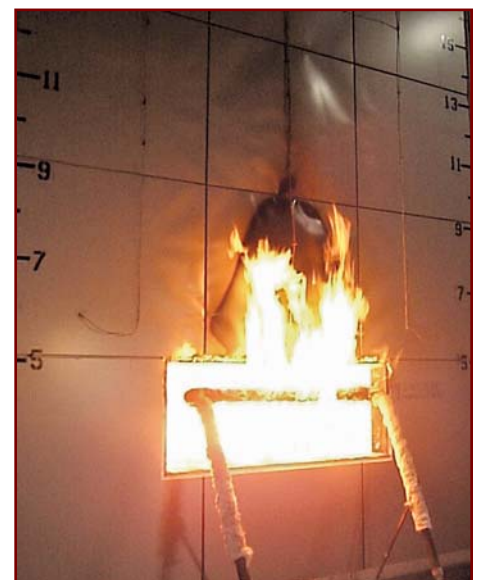
Figure 4 – NFPA 285 assembly test with NFPA 285-approved metal composite metal (MCM) veneer and ASTM C1289 Type 1 Class 2 fiberglass-reinforced ISO insulation.
