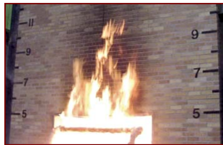
Figure 3 – NFPA 285 assembly test 285 with brick veneer wall and foam plastic insulation.
