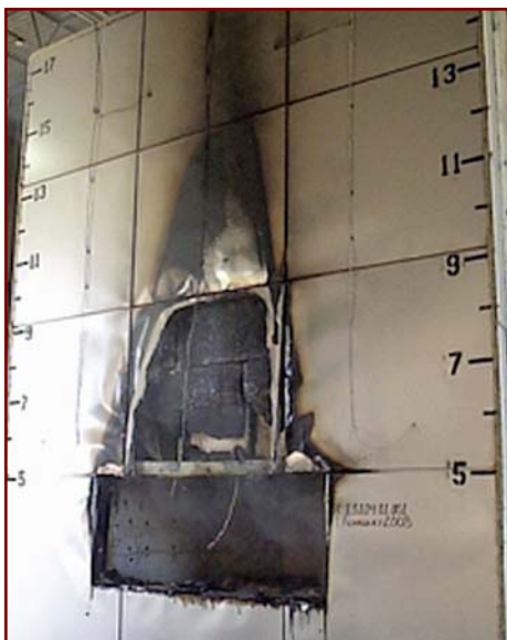
Figure 5 – NFPA 285 assembly test with an NFPA 285-approved MCM veneer and ASTM C1289 Type 1 Class 2 fiberglass-reinforced ISO insulation (post-fire view).
