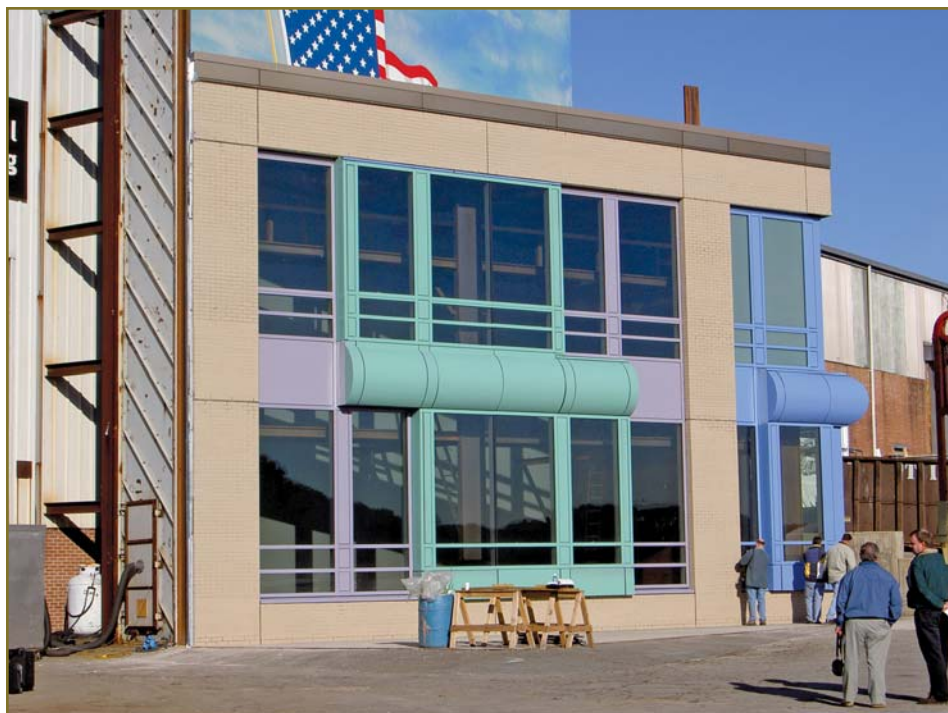
Figure 1 – Mock-up constructed at laboratory of Architectural Testing Inc.
