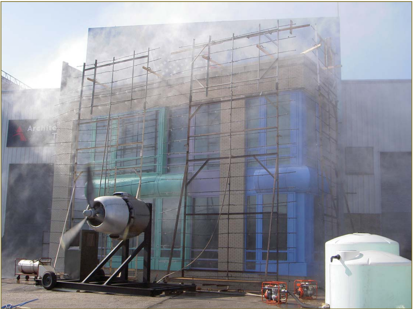
Figure 8 – Laboratory dynamic water penetration testing of mock-up window-wall section.
