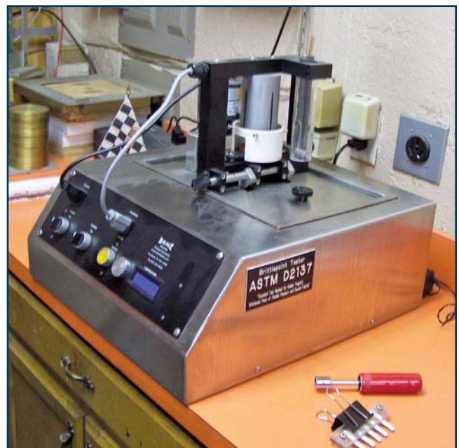
Photo 5 – Brittle-point temperature testing.
