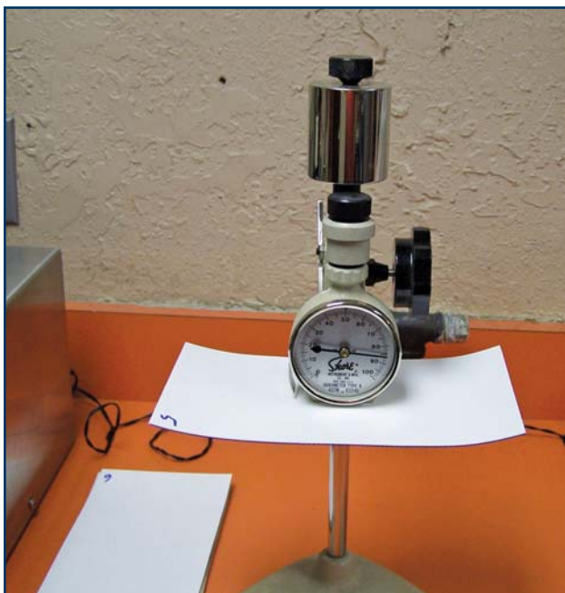
Photo 4 – Durometer hardness testing.
