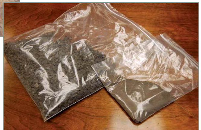
Photos 1, 2, and 3 – EPDM is removed from a ballasted system (above, left). Afterward, it is taken to the grinder (top right), and the final product results (bottom right). (Photos courtesy of ERA.)
