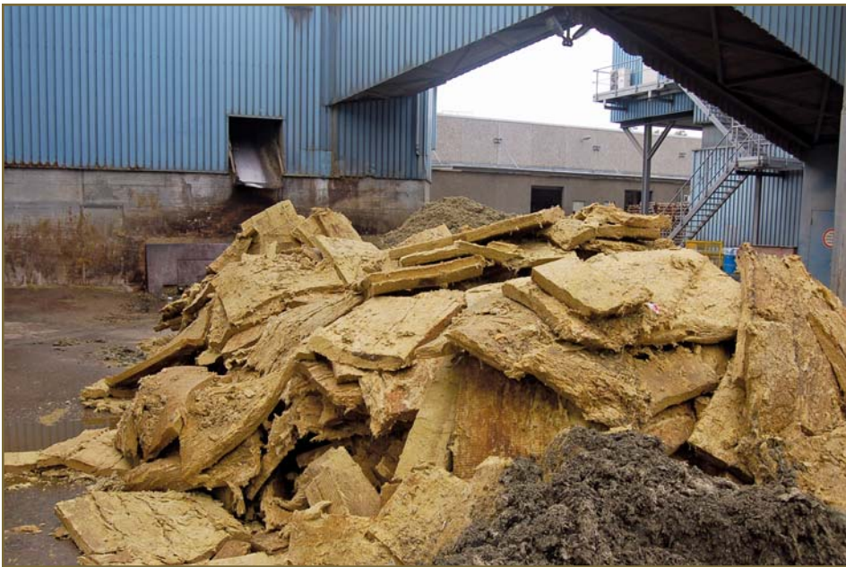
Photo 4 – Aged, used, and reclaimed stone wool for recycling.
