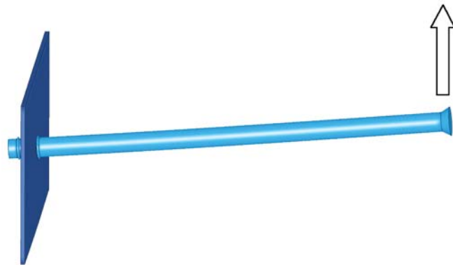
Figure 2 – Test setup and FEA model of screw-bending test.
