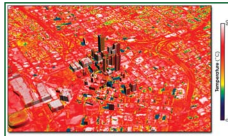
A cool roof benefits not only the building on which it is installed, but also the surrounding neighborhood. In the summer, major urban areas become heat islands, where temperatures can soar 4° to 8°F above that of the surrounding area.
