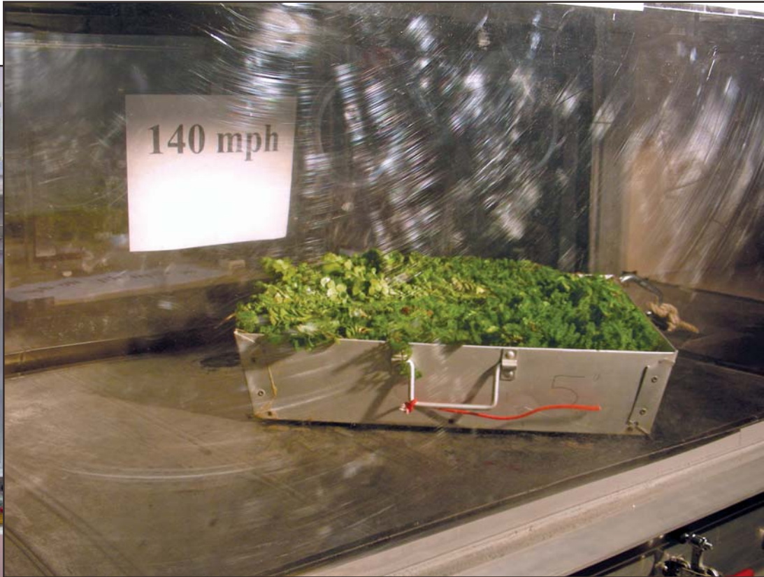
Testing at SIUE to develop prescriptive design guides for wind uplift (RP-14) for green-roof design and construction. (Photo by Kelly Luckett.)
