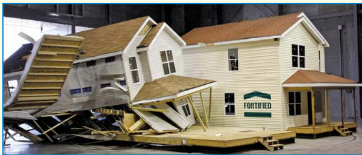
These two 1,300-sq-ft homes were constructed in the center's 21,000-sq-ft test chamber. The home on the left was built in accordance with typical U.S. building code requirements. The other home was built with certain code-plus features as outlined in IBHS's FORTIFIED for Safer Living® construction design. IBHS researchers created high-velocity wind gusts, straight-line winds reaching Category 2 hurricane strength, and wind-driven rain during the test. The traditionally built home was destroyed by winds reaching only Category 2 hurricane strength, while the FORTIFIED for Safer Living®-designed home remained intact.
