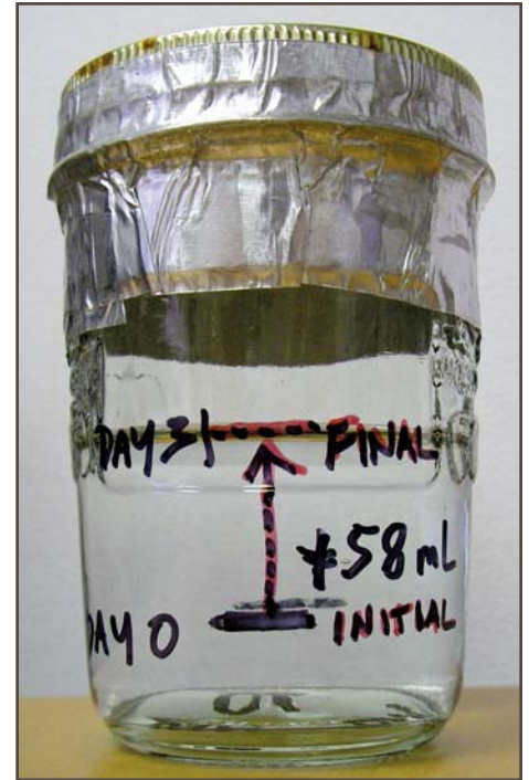
Figures 14 a (above) and b (right) – Osmotic flow testing container schematic and photograph of increase in water volume.
