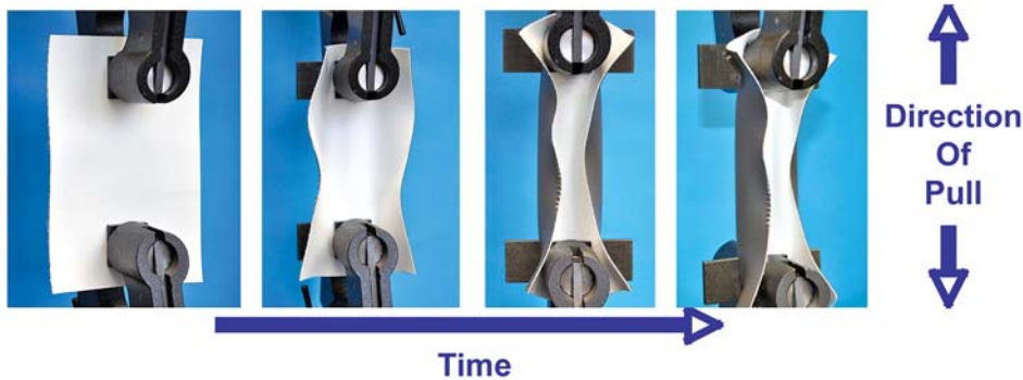
Figure 1 – Breaking strength measurement using ASTM D751. The left picture shows the membrane immediately after clamping, with no force applied. The far right picture shows the membrane just past the point of maximum force.
