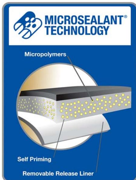
Figure 1 — Exploded view of a microsealant.
