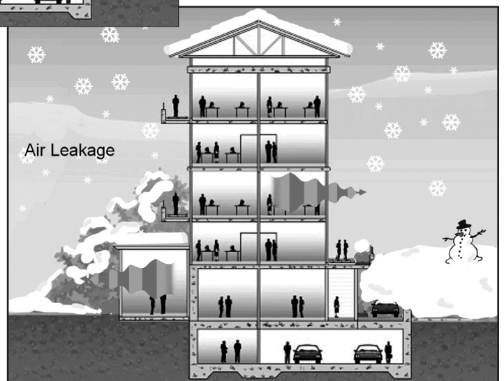
Figure 2 – Air leaking out of building.
