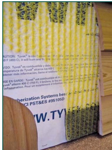
Photo 20A – Rainscreen product (Home Slicker cross section).
