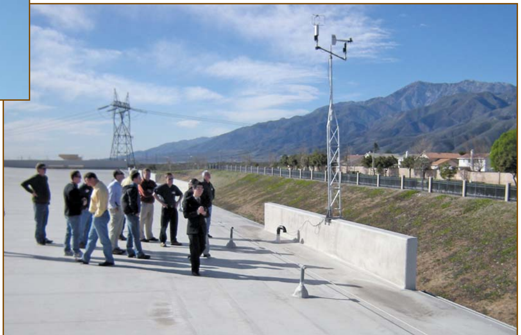
Photo 4 – Anemometers installed on mast near north Target Rialto site.
