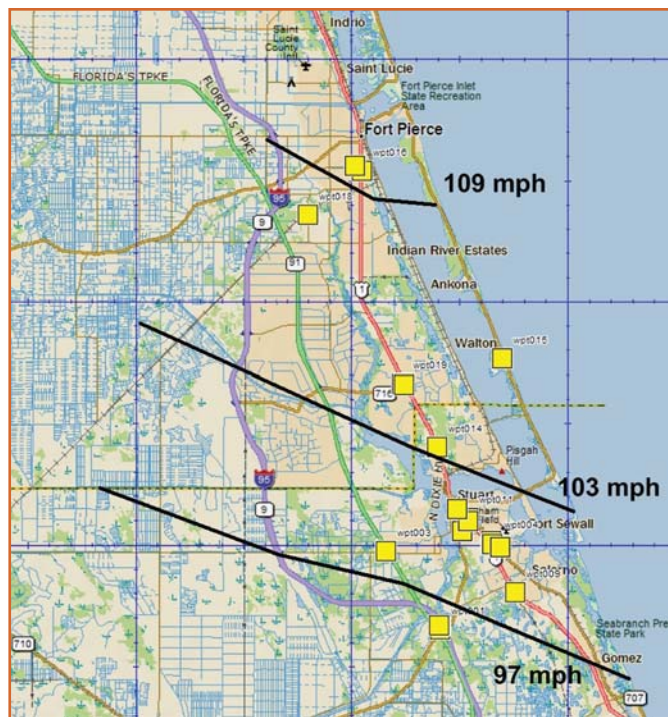
Figure 2 – Study area with Hurricane Jeanne wind contours. Yellow squares represent inspected roofs. Wind speeds are three-second gusts, 33 ft above ground, Exposure C. (Map from Topo North America 9.0, 2010, © DeLorme, Yarmouth, ME. Used with permission.)
