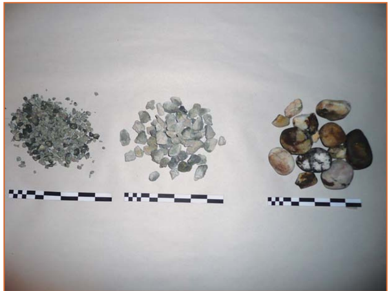
Figure 9 – Aggregate varied in average diameter between less than one-half inch and 1½ inches. Most roofs had Size 67 (nominally one-half-inch diameter).
