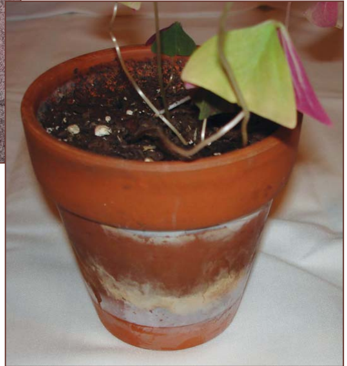
Figure 8 – Moisture mixed with the salts in a clay pot planter that was kept in the shade and formed a heavy crust of efflorescence.
