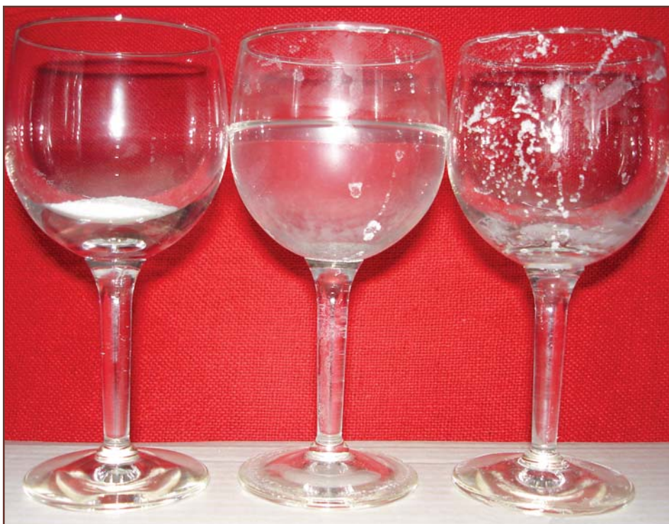
Figure 13 – Efflorescence begins with a salt deposit, combines with moisture, and then saline solution evaporates and leaves the characteristic white film.
