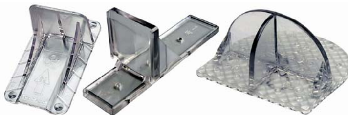
Figure 7 – Polycarbonate snow guards (below) are constructed with durable, UV-resistant plastic and are compatible with all noncopper metal roof systems. They can be attached to a roof with an adhesive or bedded in an adhesive/sealant and mechanically fastened.
