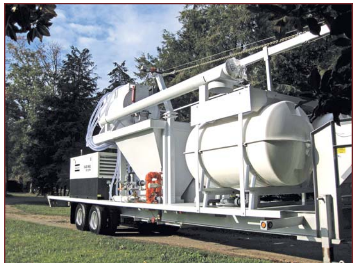
Figure 2 – LWIC batch plant equipment is designed to mix and batch LWIC at a constant, consistent mix.
