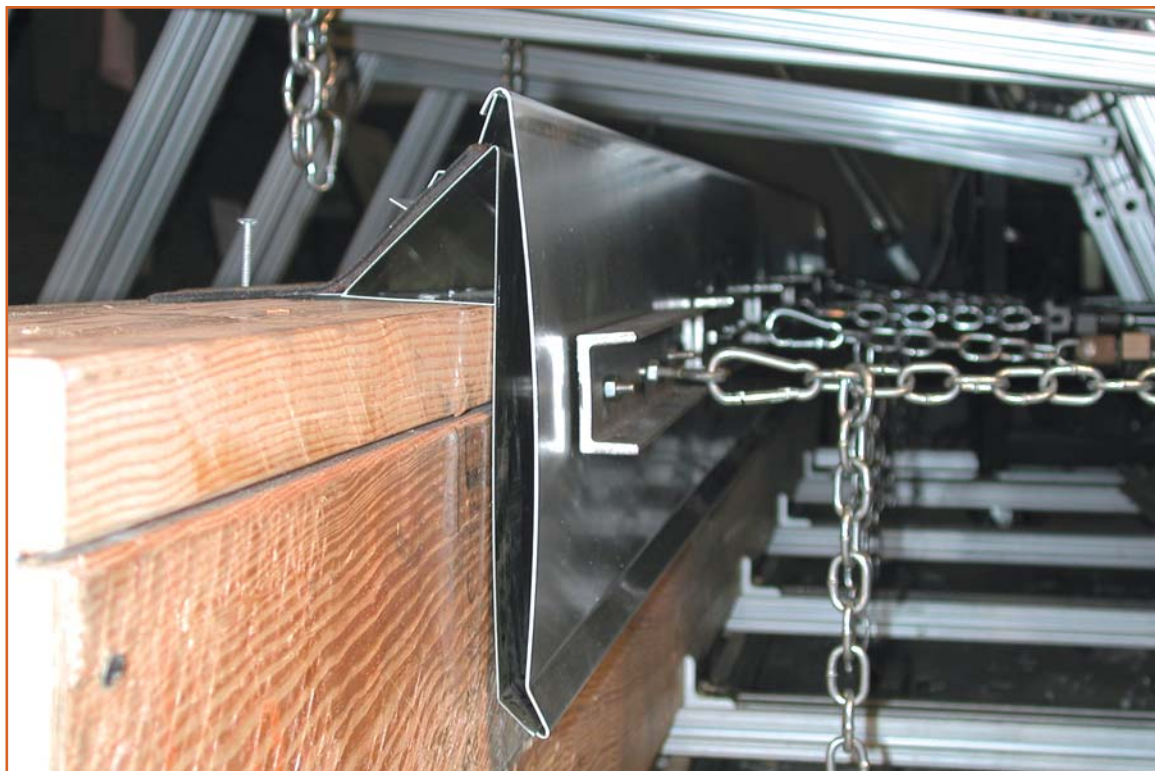
Photo 2 – This gravel stop is being tested according to the ANSI/SPRI ES-1 standard using the RE-2 test for fascia systems.
