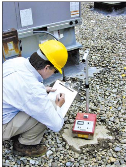
Figure 1 – A technician works with a Troxler nuclear moisture gauge (courtesy of Infra-red Analyzers).
