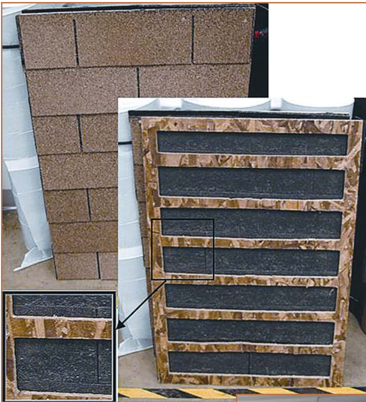
Figure 4 – Shingle layer on OSB frame with large slotted windows.
