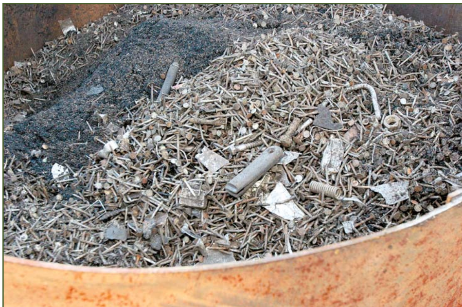
Photo 4 – Many recyclers don’t accept tear-off shingles because of nails, flashing, and other debris. Ouellette’s custom grinding device removes metal with a magnet during the first stage of a two-stage grinding process. He then recycles the scrap metal. (Photo courtesy of Dan Morrison.)
