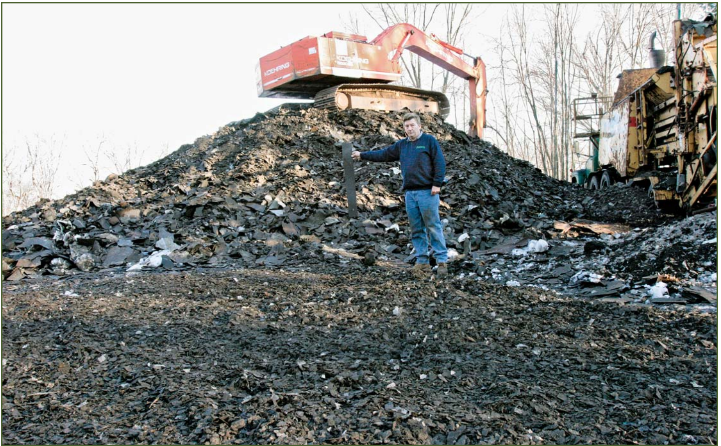
Photo 2 – If necessity is the mother of invention, Ken Ouellette is the father of asphalt-shingle recycling in Connecticut. Ouellette’s company, Incorporated Industries, grinds up used roofing shingles. The ground-up shingles are mixed with ground concrete and asphalt to make a road-paving base. (Photo, courtesy Dan Morrison.)
