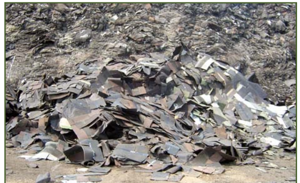
Photo 1 – Tear-offs add up. Nearly all of the 11 million tons of asphalt shingle waste produced yearly in the U.S. comes from tear-offs. Recycling programs vary from state to state. (Photo, courtesy Dan Morrison.)
