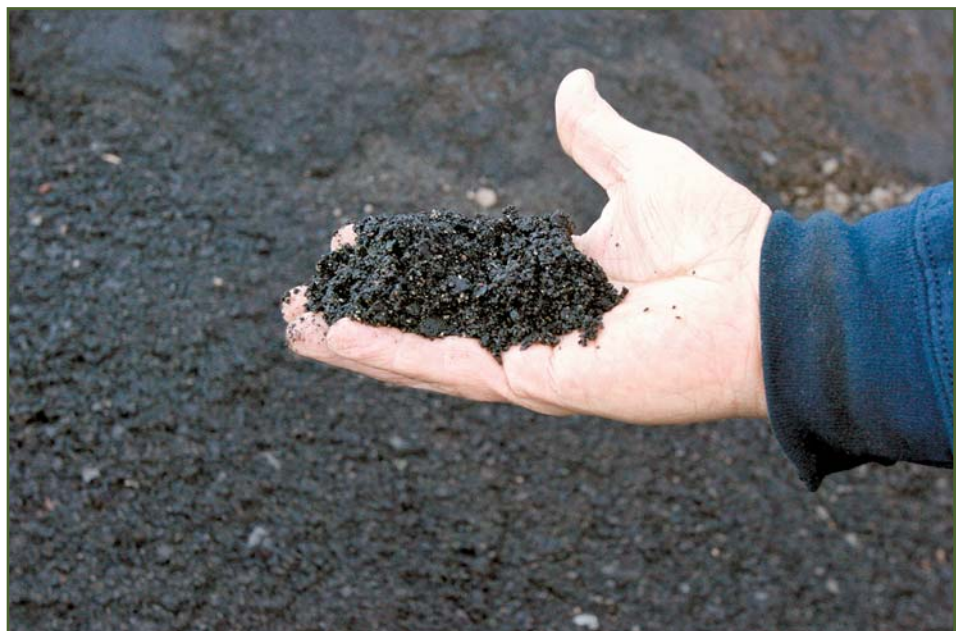
Photo 3 – A fine aggregate that contains ground asphalt shingles mixed with ground asphalt and concrete makes a great base for driveways. The mixture can be used as a temporary driveway during house construction; later, the finished driveway can be installed right on top. (Photo courtesy of Dan Morrison.)
