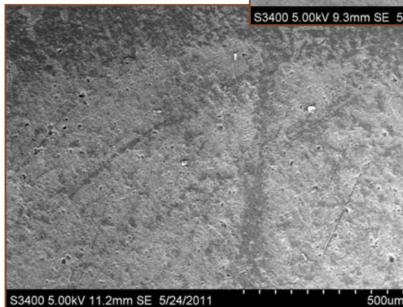
Figure 2 – 45-mil TPO at 100x magnification after 25,200 kJ-m 2 in a xenon arc weatherometer.
