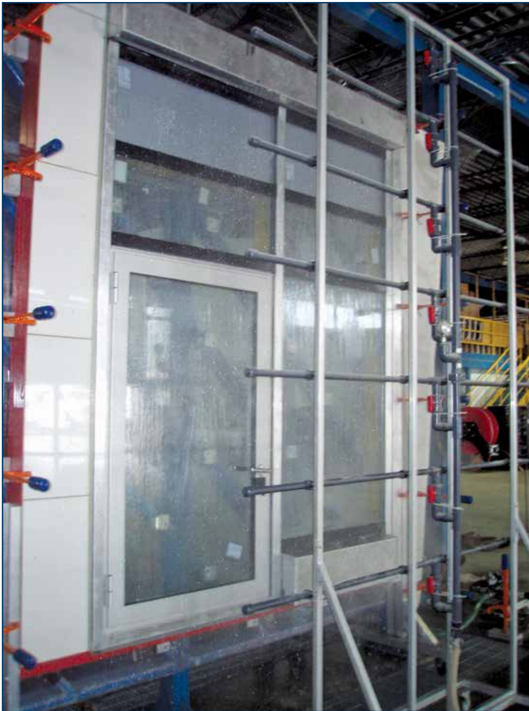
Photo 2 – Preconstruction water testing of wall mock-up used to identify problematic details prior to installation.
