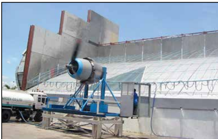
Figure 15 – Dubai International Air Terminal testing for water penetration using aircraft engine.
