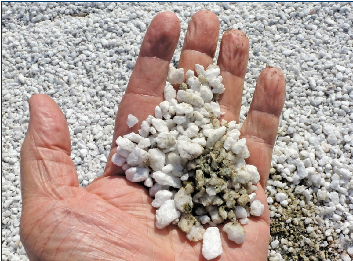
Photo 4 – A handful of rock showing the top rain-washed layer and dirty lower layer.
