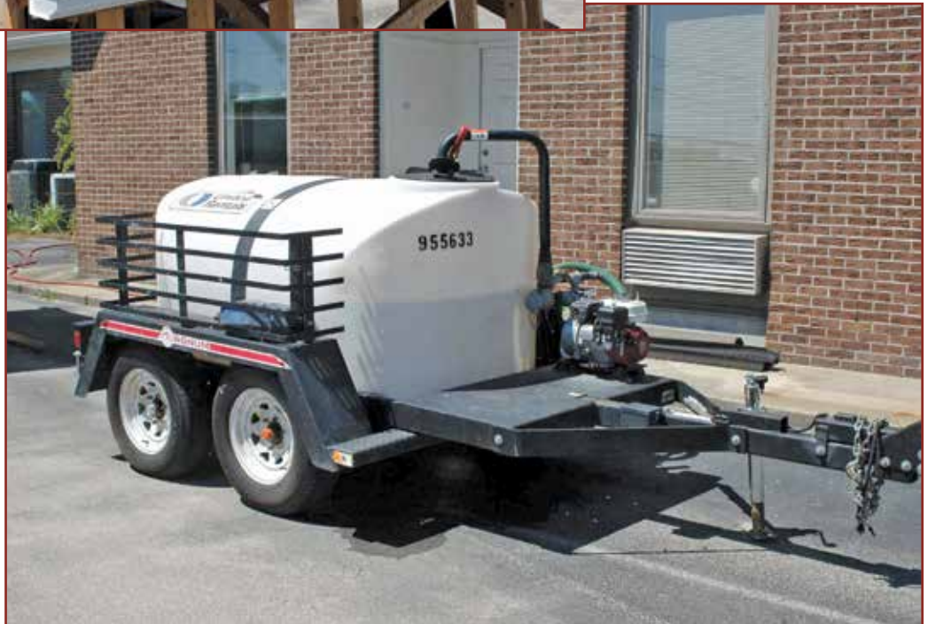
Photo 3 – Water supply was provided from a reservoir by an engine-driven pump.
