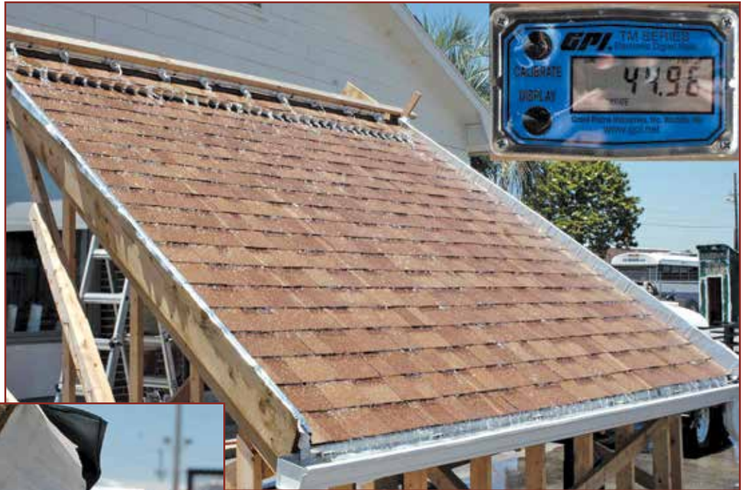
Photo 4 – View of well-distributed flow across the roof surface into the gutter. A photograph of the digital flowmeter reading is inset.
