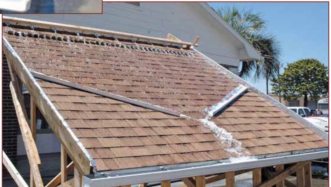
Photo 6 – Overview of the roof configuration with the diverters installed to simulate the presence of dormers. Note that the flow below the throat does not spread beyond the width of the throat.
