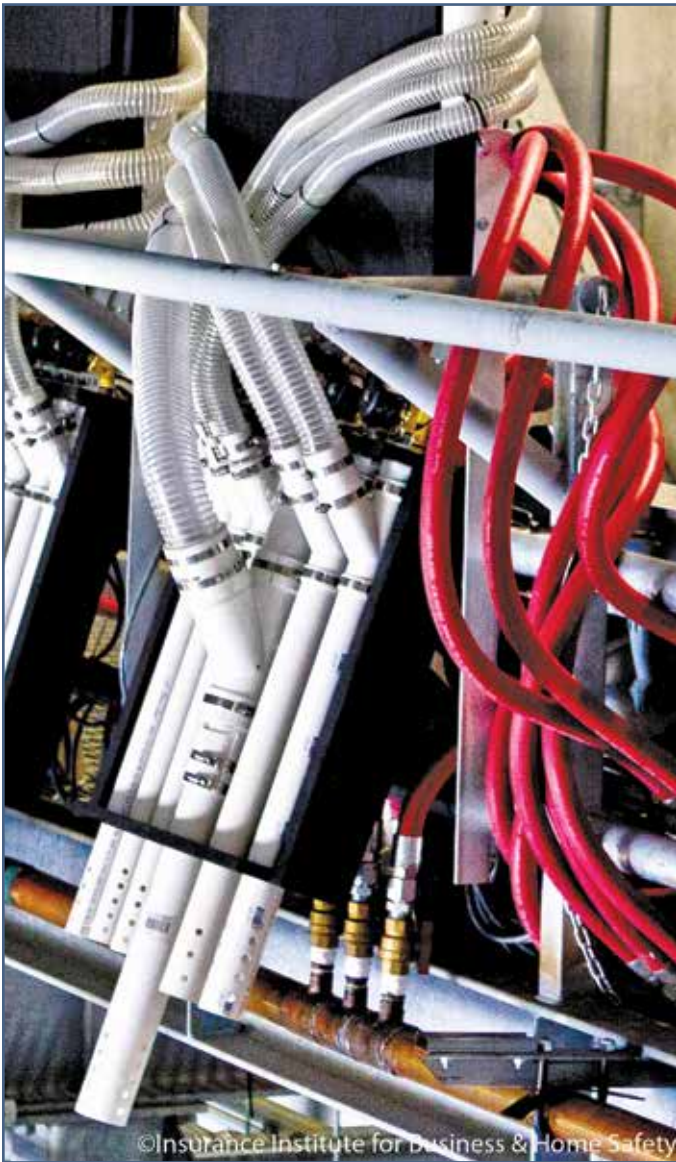
Figure 2 - One of 12 IBHS hail "pods" installed on the upper catwalk of the Research Center test chamber to create a full-scale, realistic indoor hailstorm.
