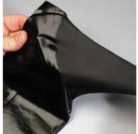
Photo 2 – Unsupported modified-bituminous flashing membrane and resulting hole from hail strike. Note: Gravel-surfaced BUR was otherwise undamaged from the hail.
