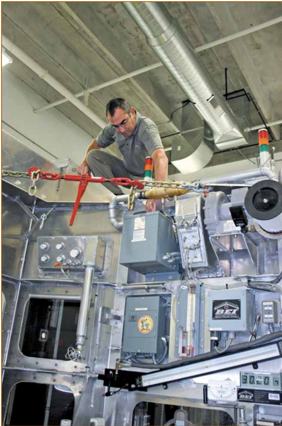
Figure 4 – Ron Tatley makes some adjustments to the Design Verification Test Chamber he developed to test the air- and watertight integrity of wall assembly mock-ups. PROSOCO photo.
