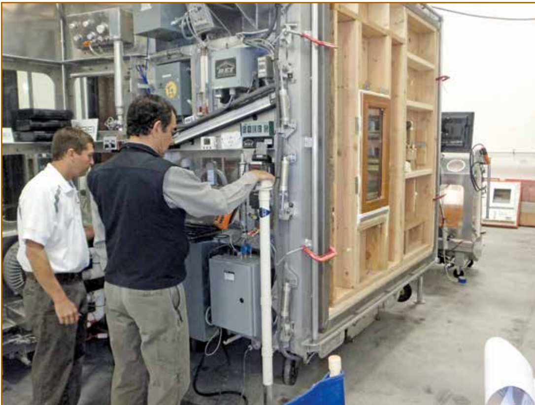
Figure 5 – Ron Tatley (right) and assistant Matt Travis test a wall assembly mock-up in the Design Verification Test Chamber. Photo courtesy of PROSOCO.
