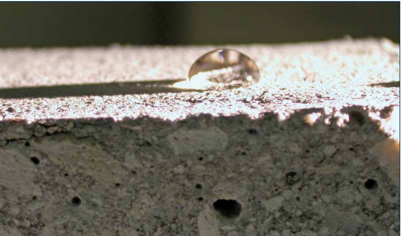
Figure 2 – An example of concrete that contains a hydrophobic admixture. Notice how the water droplet forms a tight bead and does not disperse into the concrete. Photo courtesy of Laura J. Powers of Wiss, Janney, Elstner Associates, Inc. (WJE).
