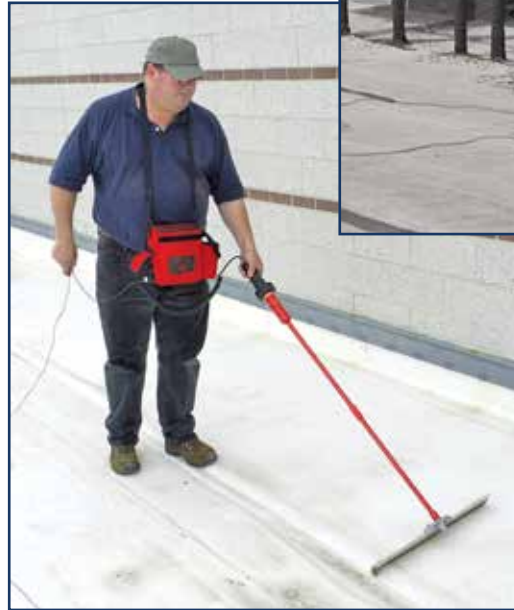
Figure 5 – High-voltage ELD is conducted by sweeping a dry membrane with an electrified brush.
