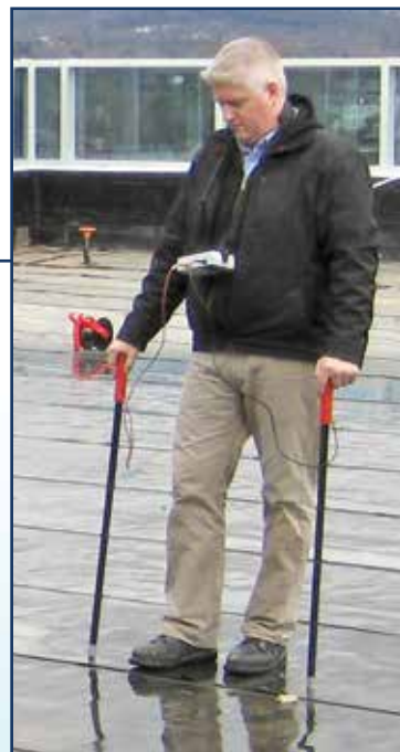
Figure 2 – Technician performing probe and trace wire method of low-voltage vector mapping on a wet membrane.
