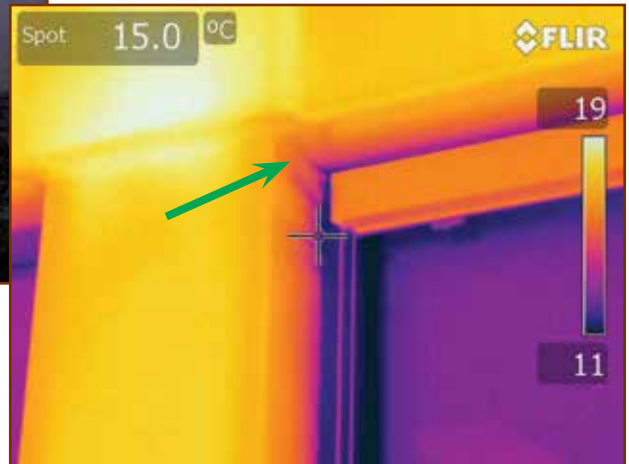
Figure 2 – Infrared (IR) image of Figure 1. Note the streaks of dark color by the arrow showing air leakage.
