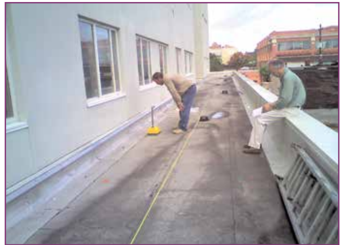
Figure 15 – Technician performing nuclear moisture testing.
