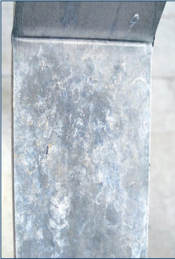
Photo 6 – Aluminum oxide on a coastal ladder. (Photo by Cris Crissinger.)
