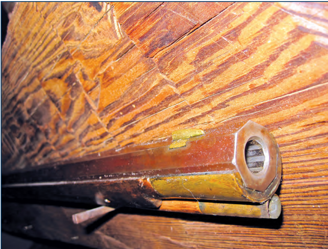
Photo 12 – Passivation (brown rust) on old rifle barrel. (Photo by Cris Crissinger.)
