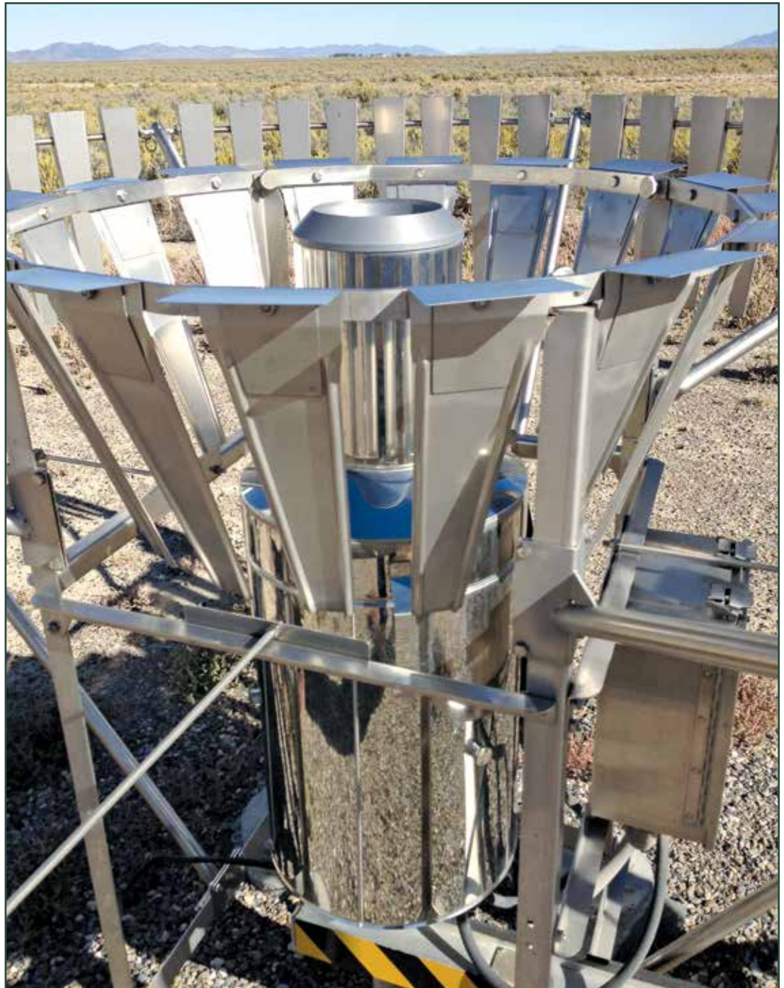
An ASOS all-weather precipitation accumulation gauge (AWPAG) at Eureka Airport, Nevada. (Photo from Wikimedia Commons.)
