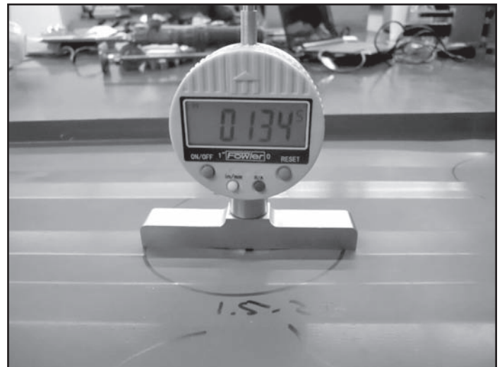
Figure 5 – Indentation measurement with micrometer.
