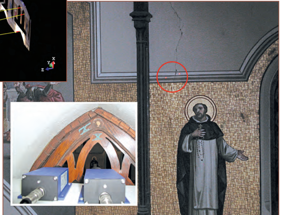
Figure 3 – The red circle highlights laser dots from two of four lasers (inset).
