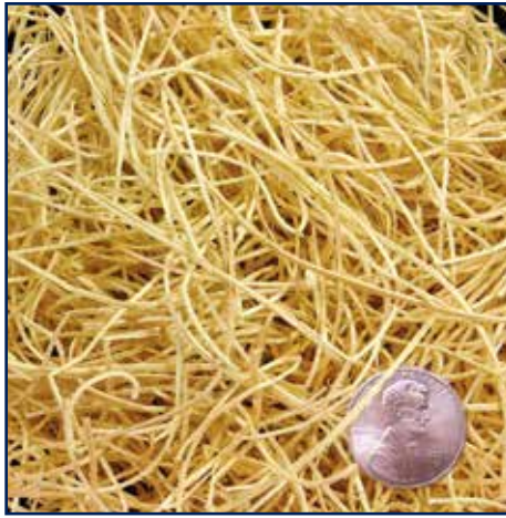
Figure 2 – The wood shavings (aspen) are known as “excelsior,” “wood wool,” and “American moss.”
