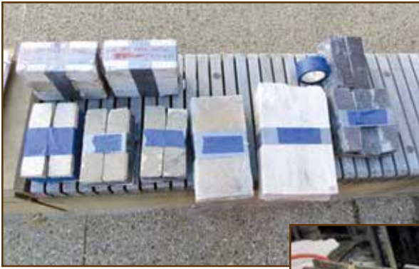
Figures 4A and 4B – Samples of each material comprising the exterior wall construction are prepared for the critical degree of saturation ( S_{crit} ) testing in a laboratory.
