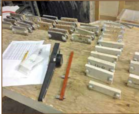
Figures 4A and 4B – Samples of each material comprising the exterior wall construction are prepared for the critical degree of saturation ( S_{crit} ) testing in a laboratory.
