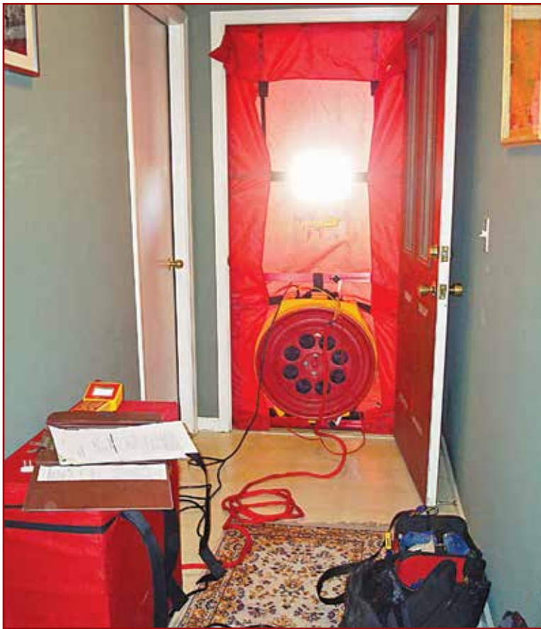
Figure 9 – This flexible, airtight, perimeter-sealed blower door is fitted with a variable-speed fan and at least two pressure gauges—one outside, one inside. The gauges measure the pressure differential across the building envelope. After closing all windows and doors to isolate the test area, the fan depressurizes the conditioned space until a pressure difference of 50 Pascals is achieved across the building envelope. (This is roughly equivalent to 0.2 in. of water column, a 20-mph wind, or 1.04 lbf/ft 2 .) If the wall leaks, more fan pressure is required to maintain 50 Pascals. That fan pressure is then converted to a measurement of air leakage usually reported as air changes per hour at 50 Pascals (ACH50).
