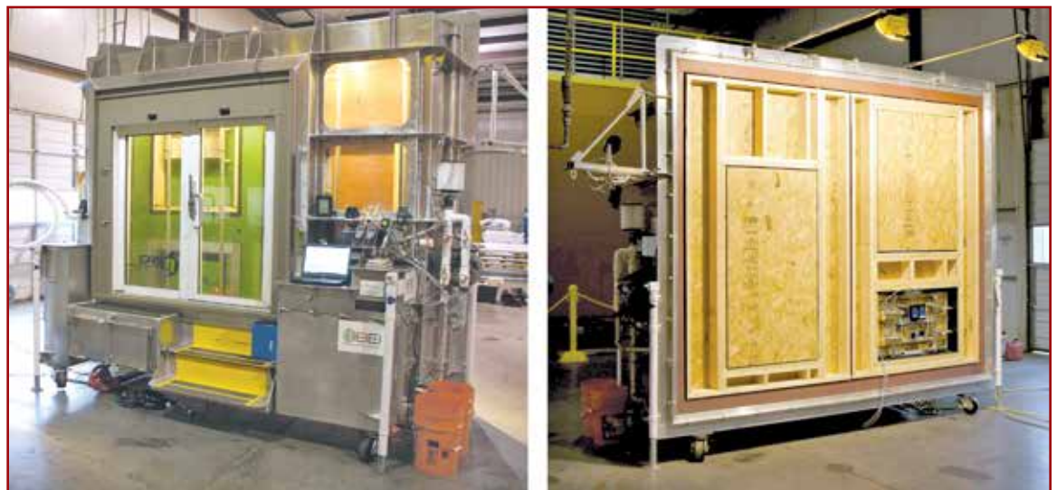
Figure 13 – The mobile DVT chamber is designed to provide testing capabilities that can simulate wind pressures and rainfalls far in excess of a 155-mph Category 5 hurricane. This is possible by use of construction detailing, methods, and materials commonly found on commercial fishing vessels. The interior is accessed by a sliding glass door produced specifically for this test chamber. When closed, the door provides visual access for testing in progress. The closed chamber has zero extraneous airflow. A laminar flow element (far too expensive for routine field testing) precisely measures airflow.
